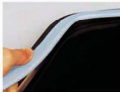
Channel Installation 1. Apply an adhesive silicone between the channel base on fixture housing to prevent slippage and stretching over time. 2. Press LED Neon-Flex™ RGB into the channel with even pressure from the beginning to the end.
