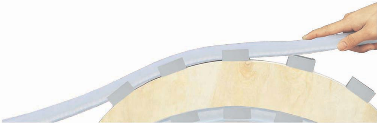
Channel Installation 1. Apply an adhesive silicone between the channel base on fixture housing to prevent slippage and stretching over time. 2. Press LED Neon-Flex™ RGB into the channel with even pressure from the beginning to the end.
